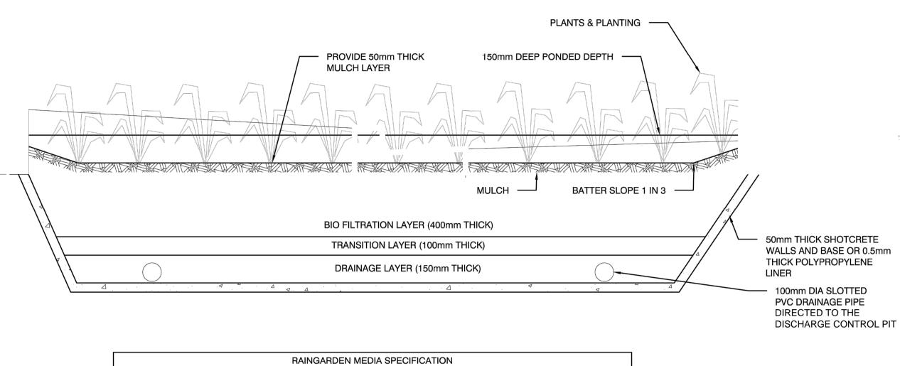
TRANSITION LAYER SPECIFICATIONS COARSE WASHED RIVER SAND OR RECYCLED - WASHED AGGREGATE 10-20mm CRUSHED GLASS EQUIVALENT BIO FILTRATION SPECIFICATION
